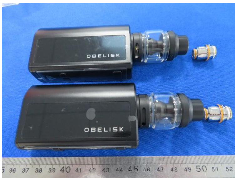
Obelisk 200 Kit with MESH Z1: 0.4ohm KA1(50-60W)/ MESH Z2: 0.2ohm KA1(70-80W)
